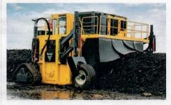
**CLEAN JOBSITE.** Operator controlled rear curtain helps maintain a clean jobsite while windrow shift is minimized by the curtain keeping material in place.
